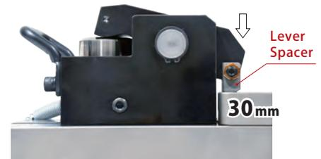
Mold Back-Plate Thickness : 30mm
